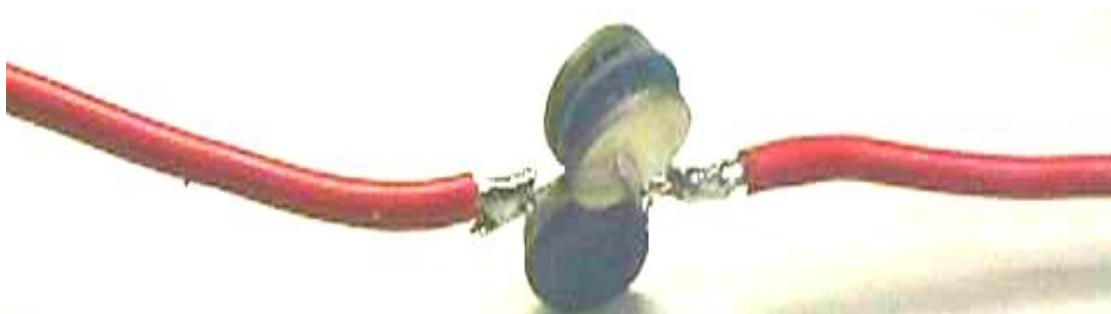
Don't forget to insulate them with a heat shrinkable tubing or with some tape. But watch out, in case that the relays fail, this item will get very hot, about 160°C (320°F ?) ! That's the way they work.
