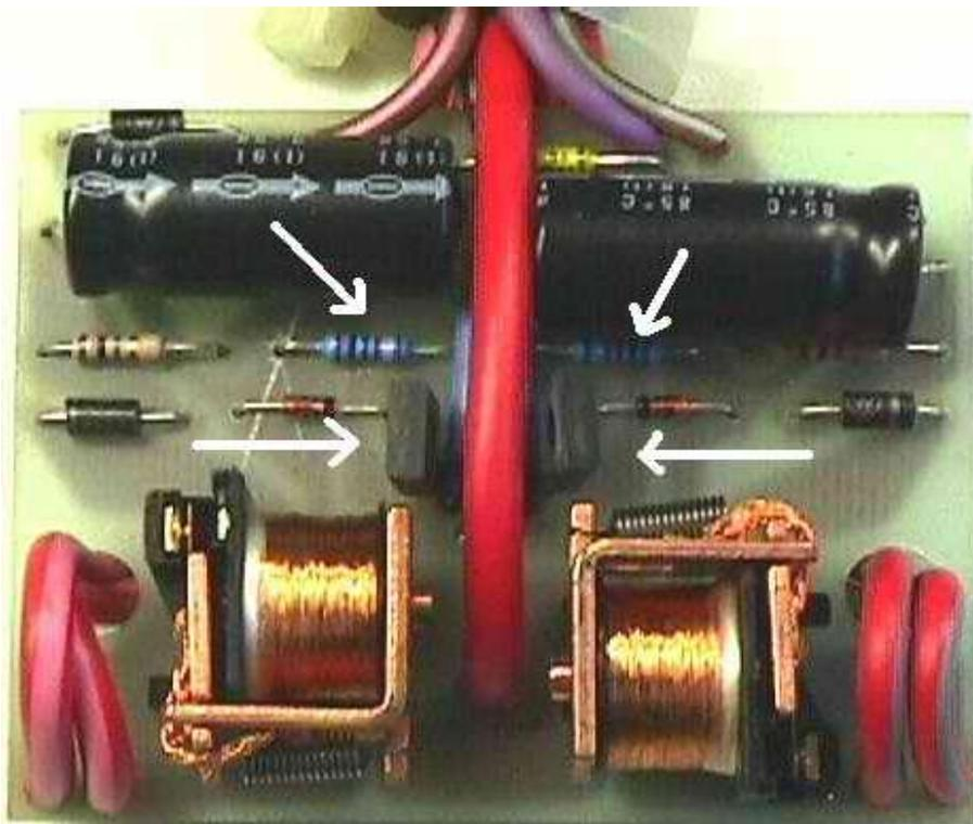
You can test your module before putting it back into the car. Take a switch with two positions (how do you call an „Um-Schalter“ in english ? A toggle-switch ?) Connect Pin 4 to +12V and the rest like following:
