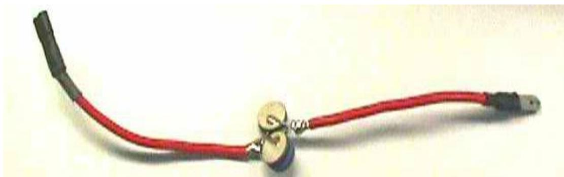
The PTCs are also called overload protection discs and sold by Siemens Matsushita. I used five parallel of the type C955 (B59955-C120-A70) with 0.8Ohm and a peak current of 5.5A.
